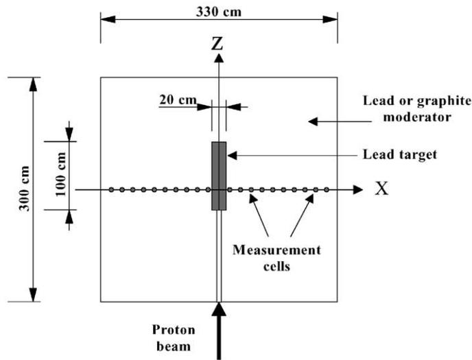
Fig. 2. XZ-cross-section of the target-moderator assemblies used in the LAHET Monte Carlo simulations. The origin of the Cartesian co-ordinate system corresponds to the centre of the assembly. (For details of the set-ups refer to the text.)
